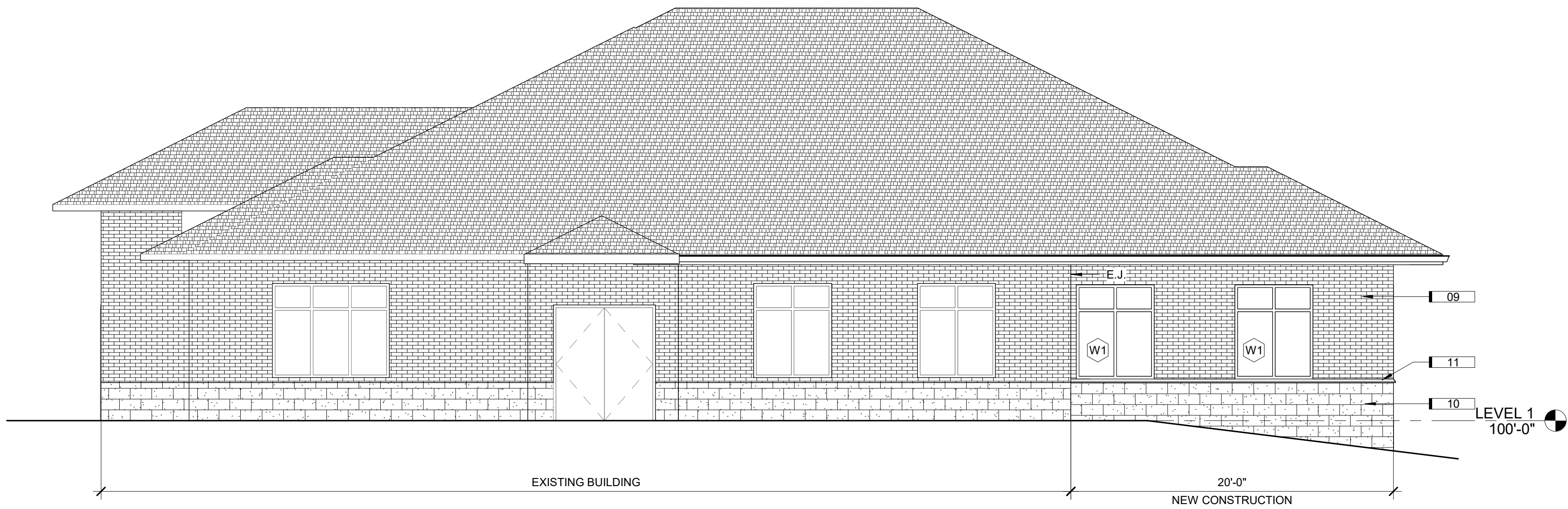
3 EXTERIOR ELEVATION - EAST 3/16" = 1'-0"
